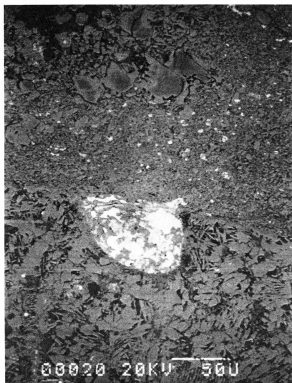
Fig. 3. Border between All-AF (lower portion) and normal Allende matrix (upper portion). Note the difference in grain-size, in the morphology of olivines and the Fe diffusion borders in the aggregate in normal Allende. Back scattered electron (BSE) picture, length is 310 \mu\text{m} .
