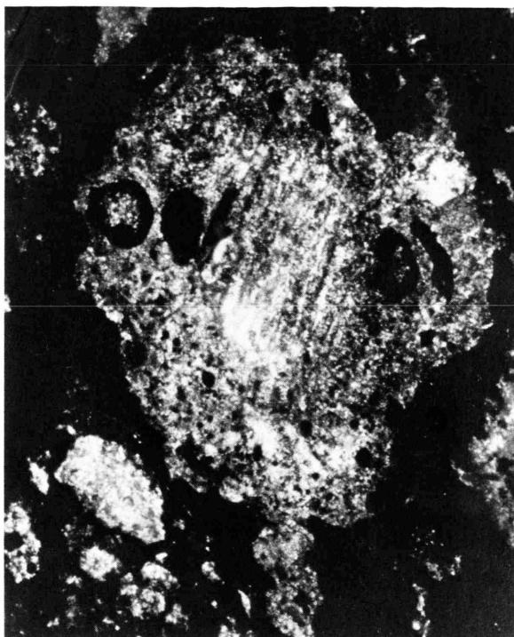
Fig. 9. Complex aggregate (AF-9) with large barred olivine (see Fig. 5) in center covered by a mantle of finer-grained aggregates rich in silicate+sulfide+metal objects (Fig. 7), some of them very large. Note lobate outline of aggregate and small fine-grained aggregates in matrix. Transmitted light picture, length is 1.3 mm.
